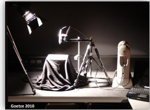
Set up for spectroscopic lab measurements using an artificial light source.
