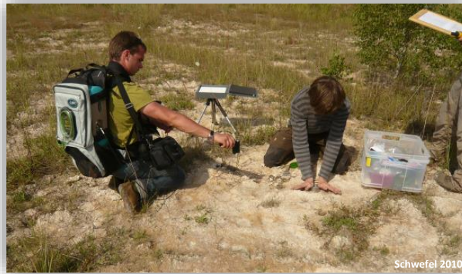
Spectroscopic field measurements and field sampling during summer 2010. The ASD FieldSpec is placed in a backpack.
